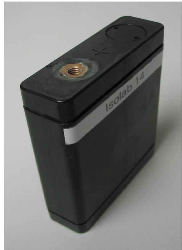
Fig. 2. Prototype cell. The terminals are on the top and bottom of the cell which has a closure on both sides of the cell and a Bunsen valve vent on one side only.
